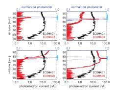
The graphs above are showing an overview of all photoelectron measurements during the summer flights ECOMA03 to ECOMA06 (red lines) compared to the results of flight ECOMA01 (black line) in September 2006, i.e. outside the polar summer period.
