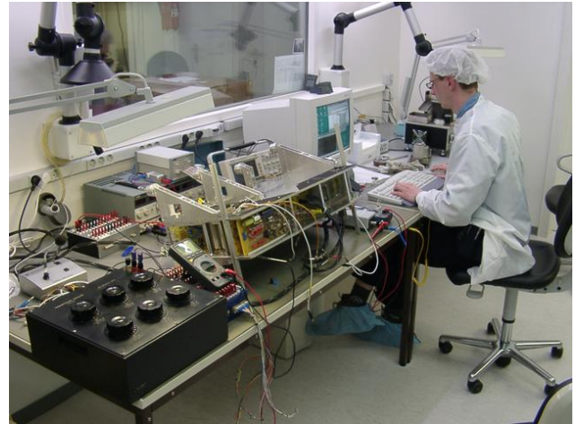
Figure 9: View into the vH&S cleanroom, during instrument calibration phase. The COSIMA electronics box is seen in the image center. On the right side: Dipl.-Ing. Andreas Koch (vH&S) at the test system.
