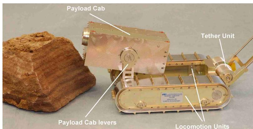
Figure 1: Generic Nanokhod rover components
