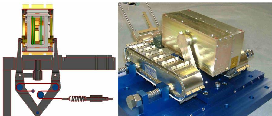
Figure 2: Left; LU conceptual holddown mechanism; Right: mock up for vibration testing (PLC released & raised)
